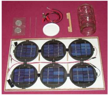
1. Cut wooden base to fit solar cells (add an extra inch or so if you are going to frame the base to protect the cells.
