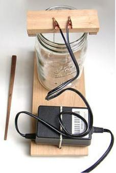
15. Wash mason jar after every use, then rinse with distilled water. Clean silver wires with scotchbrite pad to remove scale and silver crystals.
