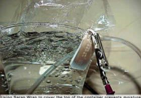
Using Saran Wrap to cover the top of the container prevents moisture from reaching the clips and becoming part of the electrolytic process
